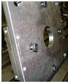
Step 1- Using the Bolts pictured above from the Fastener Bag, attach the motor to the Motor Plate. Attempt to align the terminals on the motor so that they will be positioned at 10 and 2 O'clock with the plate's longest edge horizontal. This will make wiring easier and shorten the path making it slightly more direct.
